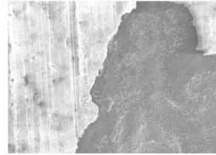
Fig. 4. SEM image of the surface of Zircaloy-4 hull sample oxidized at 600°C after 2-hr dissolution process at -0.78 V.
