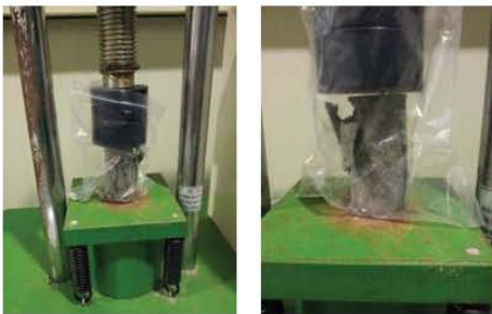
Fig. 2. Photograph for evaluation of compressive strength of cement/bottom Ash waste form.
