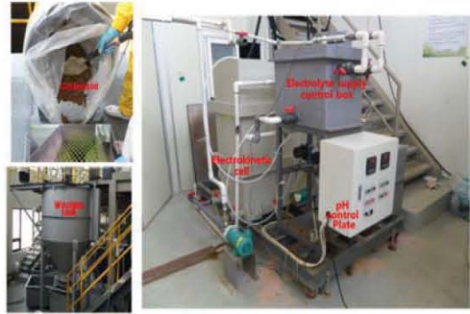
Fig. 2. Manufactured 3,000L of soil washing equipment and 540 L electrokinetic decontamination equipment.
