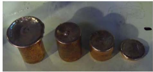
Fig. 4. Photographs of fabricated ingot with Eng. scale ingot casting equipment.
