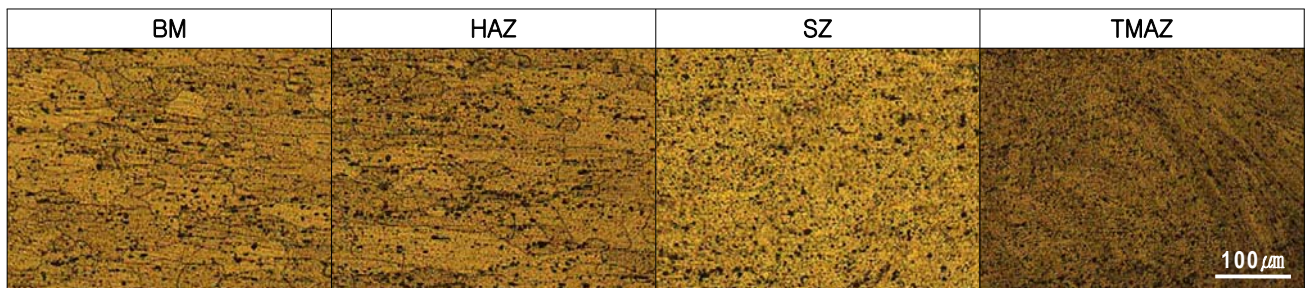
Fig. 1 Comparison of microstructures for FSWed 6061-T6 Al alloy in annealing temperature of 225°C
