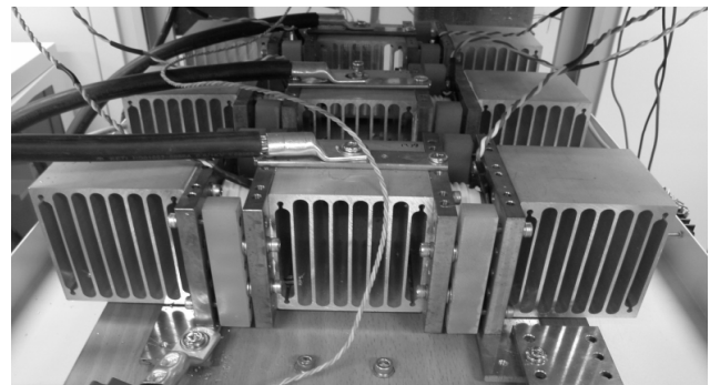
<Fig. 2> Fabrication of thyristor converter
