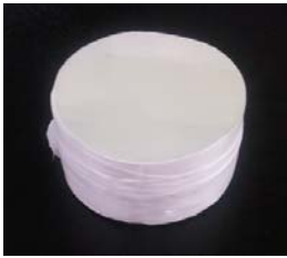
Fig 2. Grown stilbene by Bridgman technique
