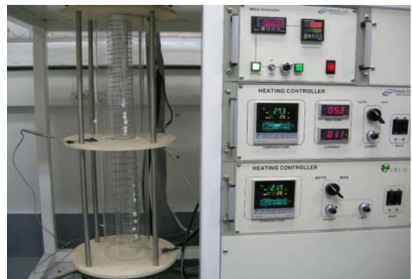
Fig. 1. Bridgman technique furnace
