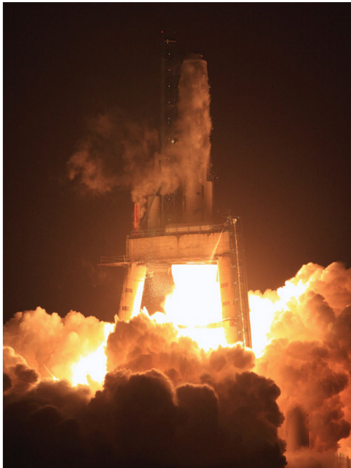
Fig. 1 Clustered engine test for Falcon 9 (credit: SpaceX)
