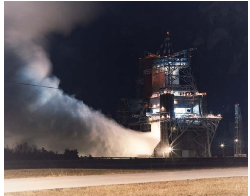
Fig. 2 SSME firing test at Stennis space center (credit: NASA)
