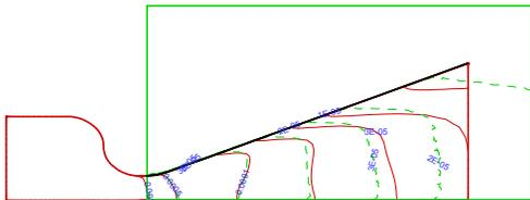
Fig. 2 Comparison of Density Contour Result between RANS and DSMC
