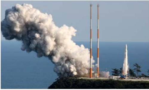
Fig. 2 Combustion gas biased by gas deflector in engine startup stage of NARO launch vehicle
