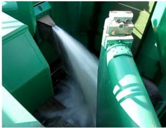
(b) Water injection test of GDCS used in Launch pad of NARO space center
