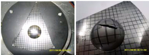
Fig. 5 Dimple and Rupture Shape of A Type Disc
