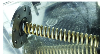
Fig. 3 Schelkin spiral; 150 mm length, 7.1 mm pitch, 49.8% blockage ratio
