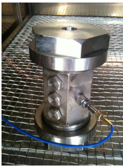
Fig. 3 The Pressure Bomb and Sample Mounting Used for Measurement of Pyrosensor Reaction
