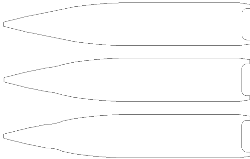
Fig. 1 Projectile Shapes for Analysis, (a) No Dent, (b) 1.5mm Dent, (c) 3.3mm Dent
