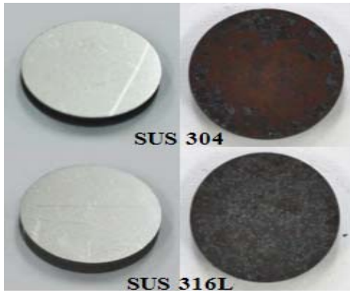
Fig. 5 Damaged surface after high temperature exposure test at 1373 K. Left is before the test, right is after the test
