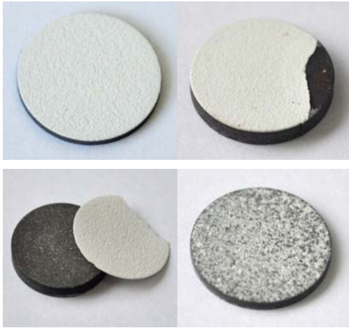
Fig. 7 Pictures of the original coating, cracked coating, separated coating, removed coating
