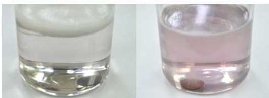
Fig. 3 Discoloration of propellant after material compatibility test (Left : Inconel 625, Right : Hastelloy C276)
