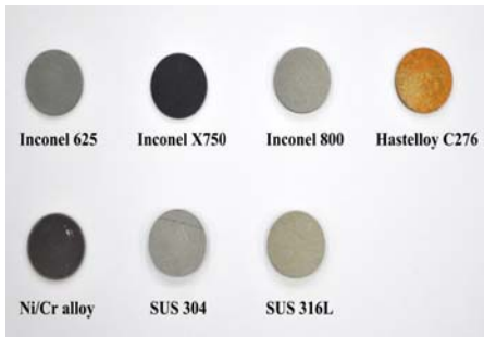
Fig. 4 Picture of materials after compatibility test
