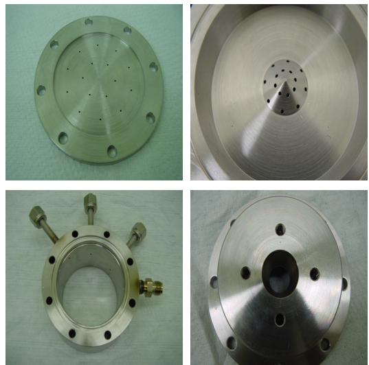
Fig. 1 Shape of injector, chamber, nozzle
