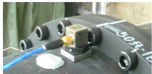
Fig. 7 Mounted vibration sensor
