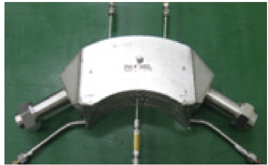
Fig. 1 air-PCM Heat Exchanger Prototype
