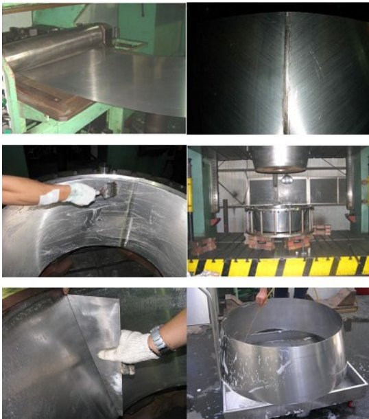
Fig. 5 Fabrication of 2nd nozzle outer jacket
