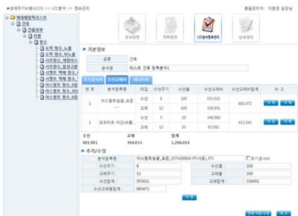
Figure 11. Repair & replacement cost - Detailed LCC analysis
