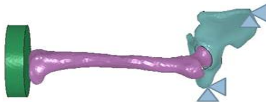
Fig. 3 Boundary condition in FE model
