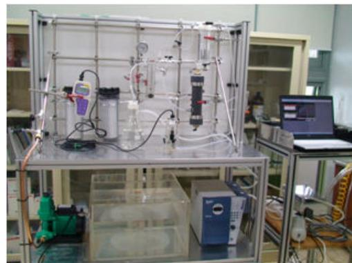
Fig. 1 Experimental devices for separation of dissolved gas
