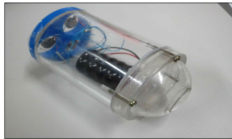
Fig. 5 Capsuled actuator constructed for experiments of linear and rotary motion
