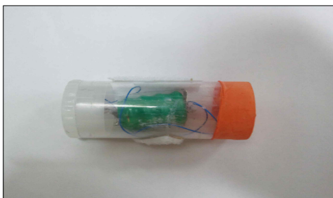
Fig. 4 Capsuled actuator constructed for experiments of linear motion
