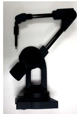
Fig. 1 Robot-Arm type 6 DOF digitizer
