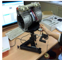
Fig. 2 Measurement of MOI for motor pump
