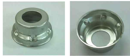
Fig. 8 The picture of cushion ring using deep drawing
