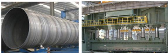
Fig. 1 Thick pipe formed by the press knife
