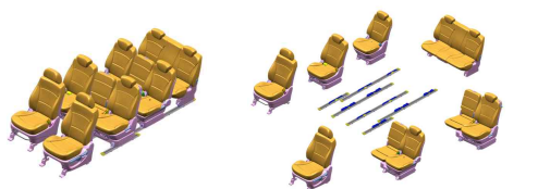
(a) Seat Lay-out (b) Arrangement of Sliding Seat Fig.1 Sliding Seat of Van
