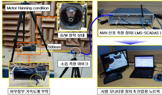
Fig. 2 Experimental Set-up for the NVH test
