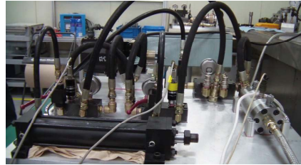
Fig. 5 Experimental setup for spool-sleeve performance testing
