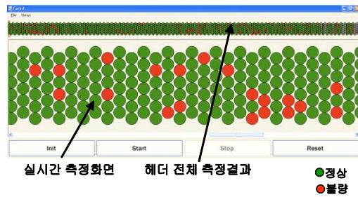
Fig. 4 Result of water evaluation at real cooling header
