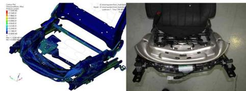
Fig. 2 Comparison of the result of sled test and simulation
