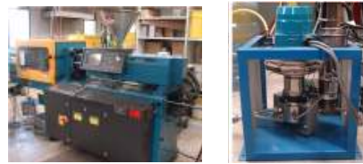
Fig. 1 Injection molding machine & gas control units
