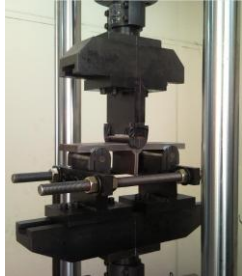
Fig. 2 Test specimen and 3-point bending jig
