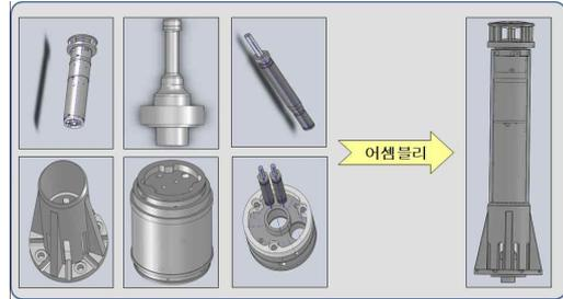
Fig. 1 3-D Modeling of weather detector
