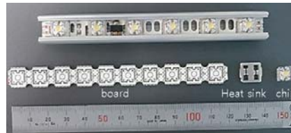
Fig. 1 Main components of a LED package
