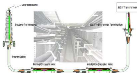
Fig. 1 Normal straight joint and insulation straight joint
