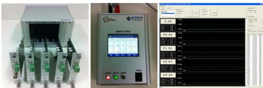
Fig. 2 Integrated monitoring system(analog signal processors, main board, signal processing Program)
