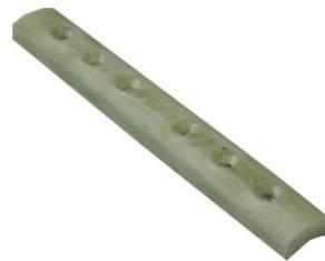
Fig.1 Fabricated composite bone plate
