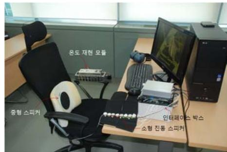
Fig. 1 Implemented Pseudo aural-sensation display system consisting of vibro-tactile speakers and thermal display module
