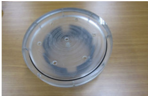
Fig. 3 Device for gathering dissolved gas separated from 2 membranes
