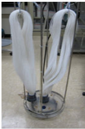
Fig. 2 Experimental device with 2 membranes for separation of dissolved gas
