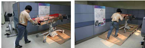
Fig. 4 Drivability Tests using a Shower Carrier with an Human Dummy on a Sloped Surface
