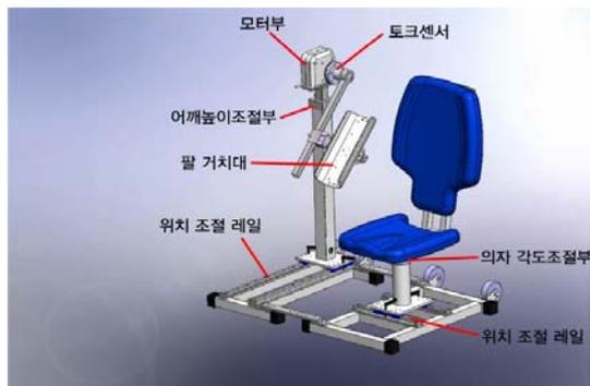
Fig. 1 Biofeedback control motion system
