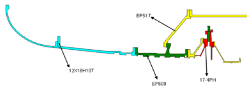
Fig.2 Simplified 2D axisymmetry casing model
