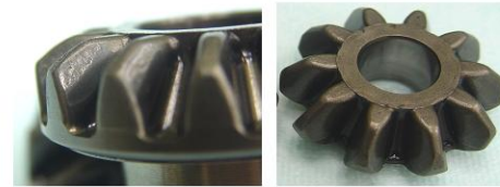
Photo. 3 Photograph of Bevel gear set after Endurance test (Sample #1 m3.991)
