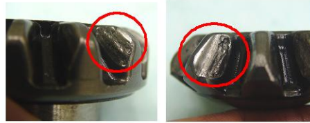
Photo. 2 Photograph of Bevel gear set after Endurance test (Sample #1 m4.298)
