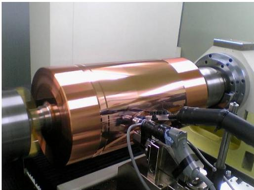
Fig. 1 Experimental Equipment (Drum lathe)
