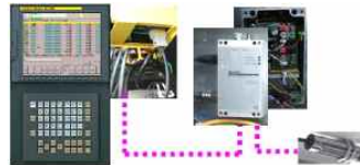
Fig. 1 Connection RFID for Fanuc CNC
