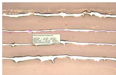
Fig. 2 Bad quality printing result example
