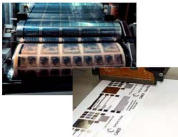
Fig.1 Printing method for printed electronics: (a) Gravuring; (b) Inkjet printing.
