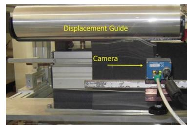
Fig. 2 Camera for lateral displacement detection
