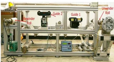
Fig. 1 Roll-to-roll simulator
